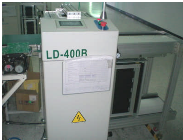
SMT Automatic material loading machine
